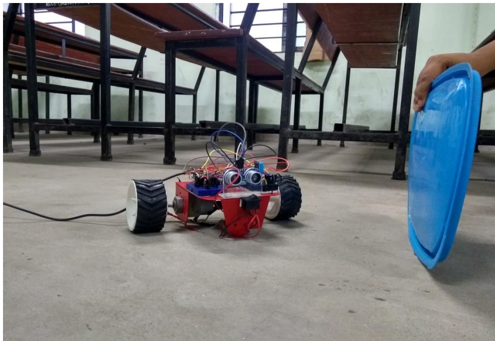
Fig 16. The robot after detecting an obstacle changes direction.
