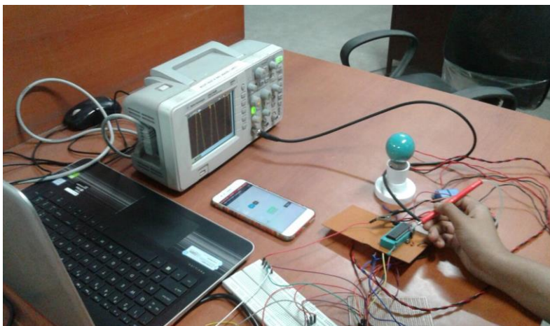
Fig 12b: Bit pattern observed in DSO when switch is on in App
