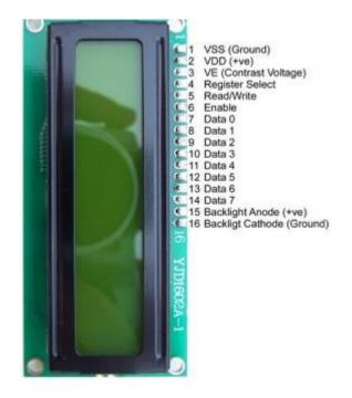
Fig 8 :- A 16x2 LCD display with pin layout
