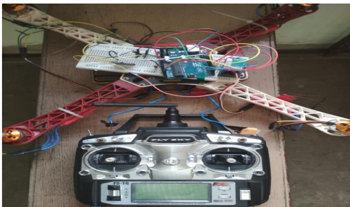
Figure 6: Arduino as flight controller
