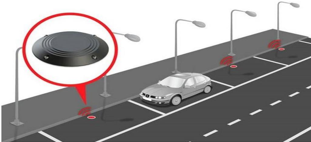
**Identification between Animals and Vehicle**:-It may happen that the light may light up if any animal passes over the sensor so a method of prediction based on the speed of movement will be enabled which will calculate the speed and depending on that the light will lighten up and in addition to that error will be less as vehicle have greater surface area and hence have higher probability of triggering the sensors.
