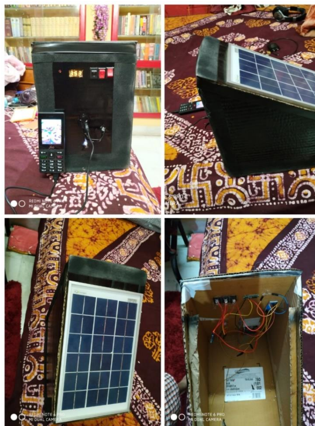
Fig. 14 Hardware implementation of the device
