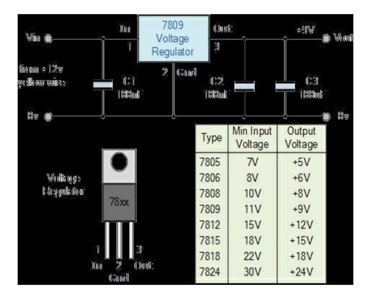
So suppose we want an output voltage of +9 volts from our PSU bench power supply, then all we have to do is connect a +9v voltage regulator to the +12V yellow wire. As the PSU has already done the rectification and smoothing to the +12v output, the only additional components required are a capacitor across the input and another across the output.
