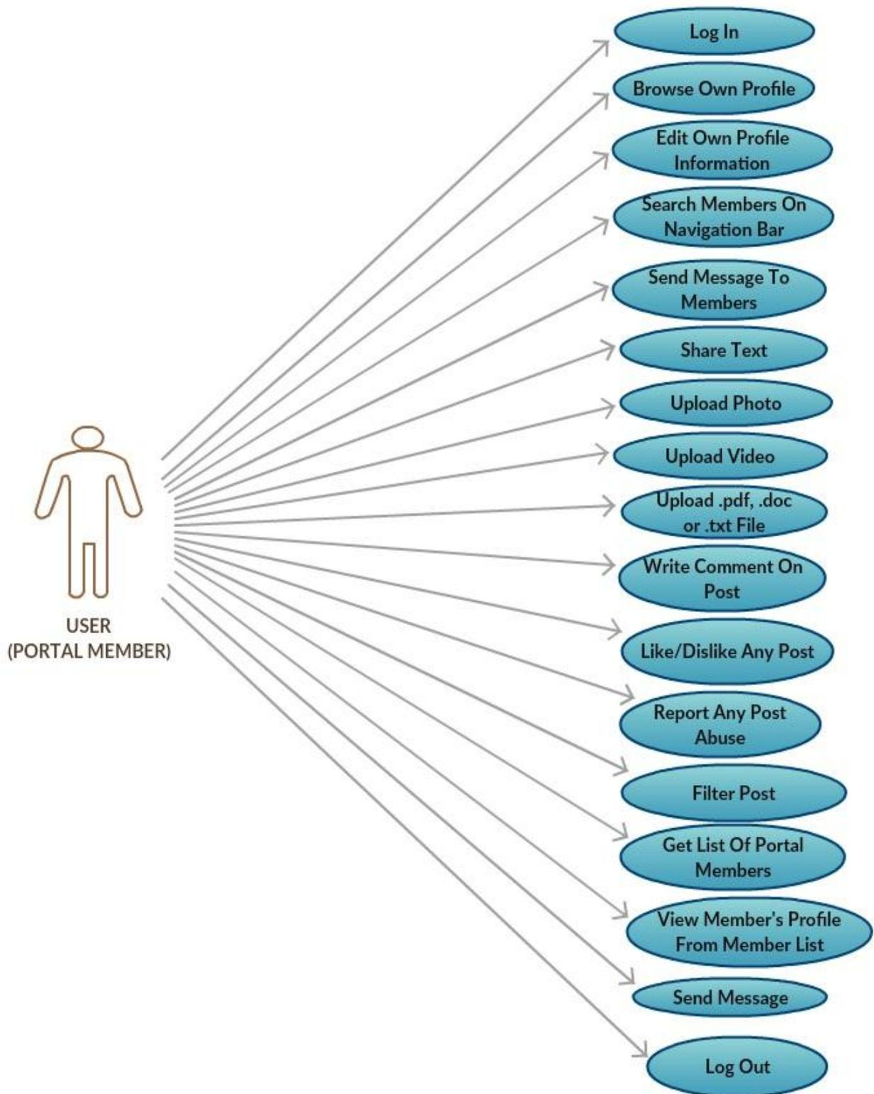
**FIG: USE CASE DIAGRAM OF AFTER LOGIN PAGE**
